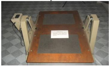
This apparatus is used to assess subject's optimal ability to utilize bilateral motor coordination required for balancing , and lateral motor control required for peak sports performance.
