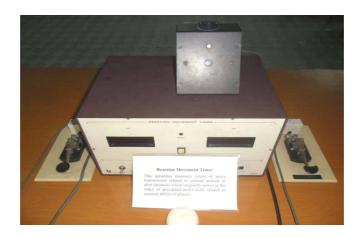
This apparatus measures extent o nerve transmission related to cortical arousal in alert situations which originally serves as the index o perceptual motor-skills related to reaction ability o players.
