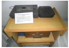
This apparatus assesses the changes in evoke potential of the muscles as index of arousal modulation in the peripheral nervous system (PNS). In the field of sports, this instrument is used for the purpose of regulation of muscle tension, employing by feedback training.
