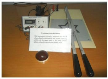
This apparatus primarily measures the level of eye-hand coordination and motor learning ability of the upper part of the body of the players related perceptual motor skill.
