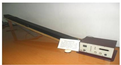
This apparatus measures the visual anticipation ability of the player in static condition. This is an index perceptual motor skill required in anticipation of time – lapse before the onset of stimulus and the perceptual – motor conditioning (eyehand coordination) required for appropriate reaction.
