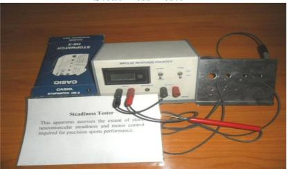
This apparatus assesses the extent of static neuromuscular steadiness and motor control required for precision sports performance.
