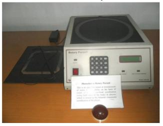
This is an apparatus aimed at measurement of motor learning ability on basis of extent of bilateral eye-hand coordination (using both sides of the body) in players, which is termed as the bilateral visuomotor coordination of the players.
